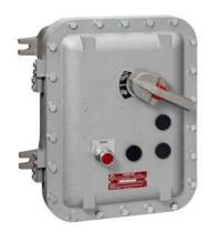
Non-reversing motor starter, Size 1, Three phase full voltage, Solid-state overload relay, OLR amp range 10-40A, 110V 50HZ / 120V 60HZ coil, Combination type, 60A non-fused disconnect Encl. NEMA type 4X Fiberglass Water/dust tight noncorrosive, Standard width enclosure
