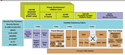
Core Complex (CPU, L2 and Frontside CoreNet Platform Cache) Basic Peripherals and Interconnect
