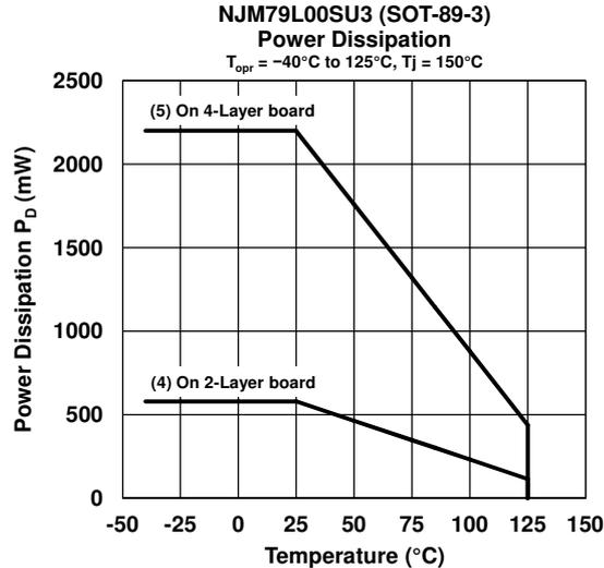
(4) 2-Layer: Mounted on glass epoxy board (76.2 mm × 114.3 mm × 1.6 mm: based on EIA/JEDEC standard, 2-layer FR-4).
