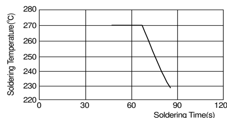
[Allowable Reflow Soldering Temperature and Time]
