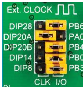
Figure 4-7: Position of the jumpers for DIP20A
