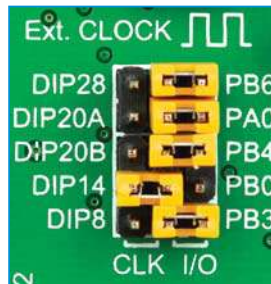
Figure 4-9: Position of the jumpers for DIP14
