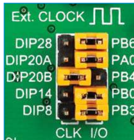
Figure 4-8: Position of the jumpers for DIP20B
