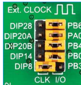
Figure 4-10: Position of the jumpers for DIP8
