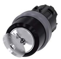
RONIS key-operated switch, 22 mm, round, plastic with metal front ring, lock number SB30, with 2 keys, 2 switch positions O-I, latching, actuating angle 90°, 10:30h/13:30h, key removal O, possible special locks: SB31, 421, 455, with laser labeling, upper case
