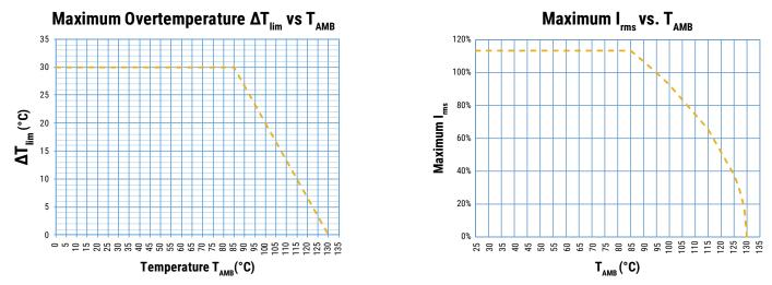
*T*<sub>AMB</sub> is the maximum ambient temperature surrounding the capacitor or hottest contact point (e.g. tracks), whichever is higher, in the worst operation conditions in °C.
