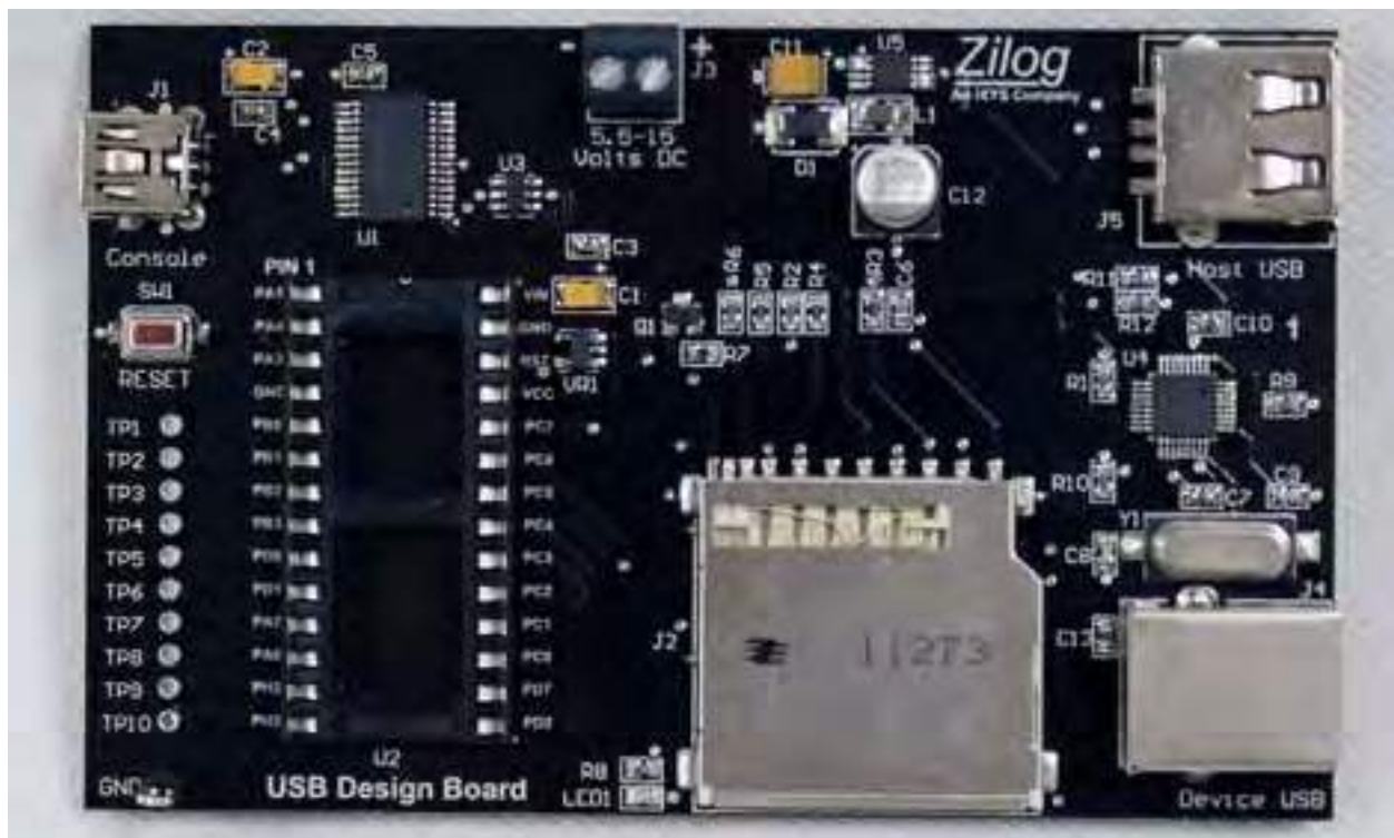
Figure 1. The Mini-Z USB Design Board
