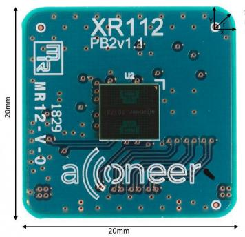
x=y=2.05mm r = 2.9mm PCB thickness: 0.9mm
