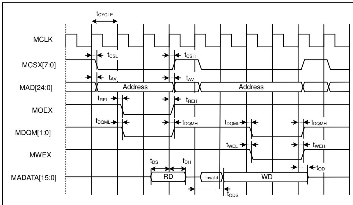
**■ Multiplexed Bus Access Asynchronous SRAM Mode**
