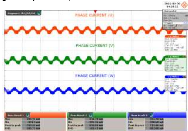
Figure 25 – Phase Current at 30 W Load.
