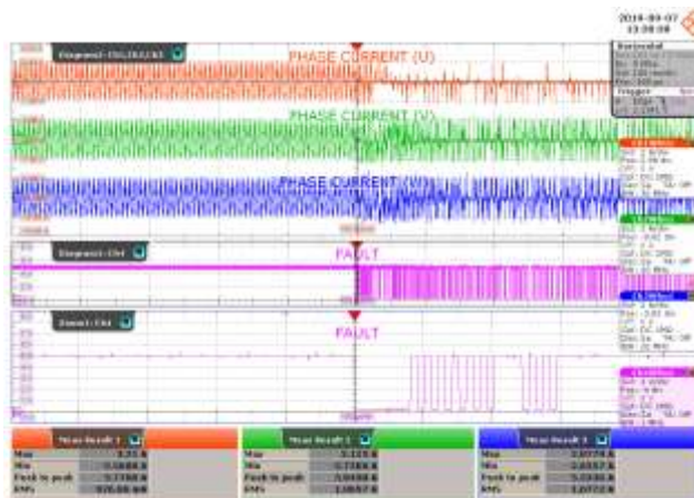
Overload Test >200 W
