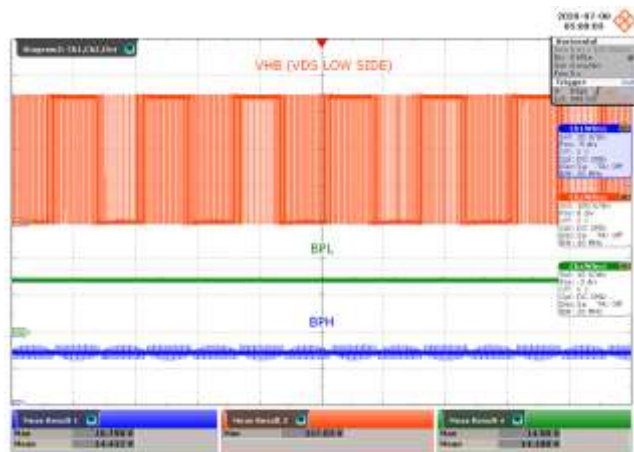
Figure 35 – BPL and BPH Signals at 200W Load.
