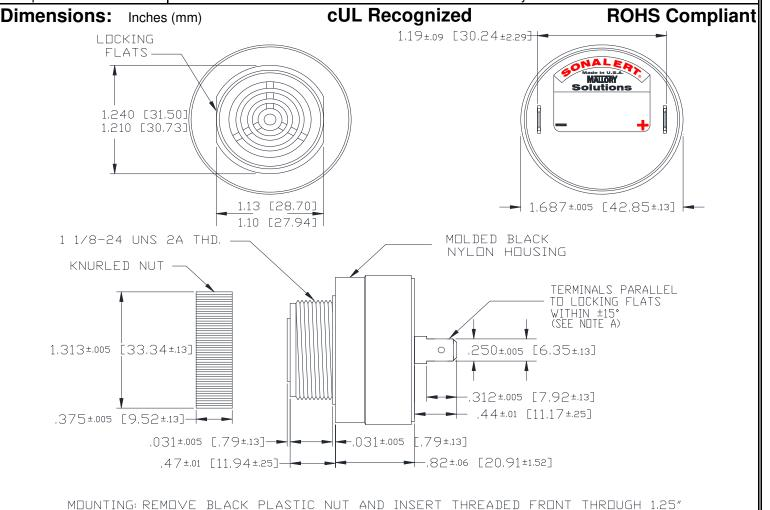
HOLE PUNCHED IN PANEL, IF DRIENTATION IS NEEDED, NOTE LOCKING FLATS
