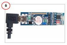
LED D1 of CY3240 USB-12C Bridge and LEDs D3 and D2 of demo board light up.
