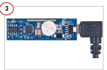
Connect the USB A to Mini B cable and the bridge to the PC. LED D2 (green) lights up.
