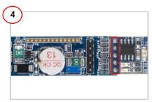
Plug in the I2C slave demo board to header J3 of the bridge board.
