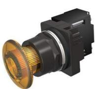
30mm BlackMax, Epoxy Coated Corrosion Resistant Complete Metal Unit Illuminated Push-Pull Operator Transformer type, 120V AC Incandescent Lamp Mushroom Head Cap Small 1 3/4" (44.5 mm) Plastic, Amber 2 Position Maintained, Pull-to-Release UL Listed, CSA Certified NEMA 1,3,3R,4,4X,12,13 & Automotive Standards
