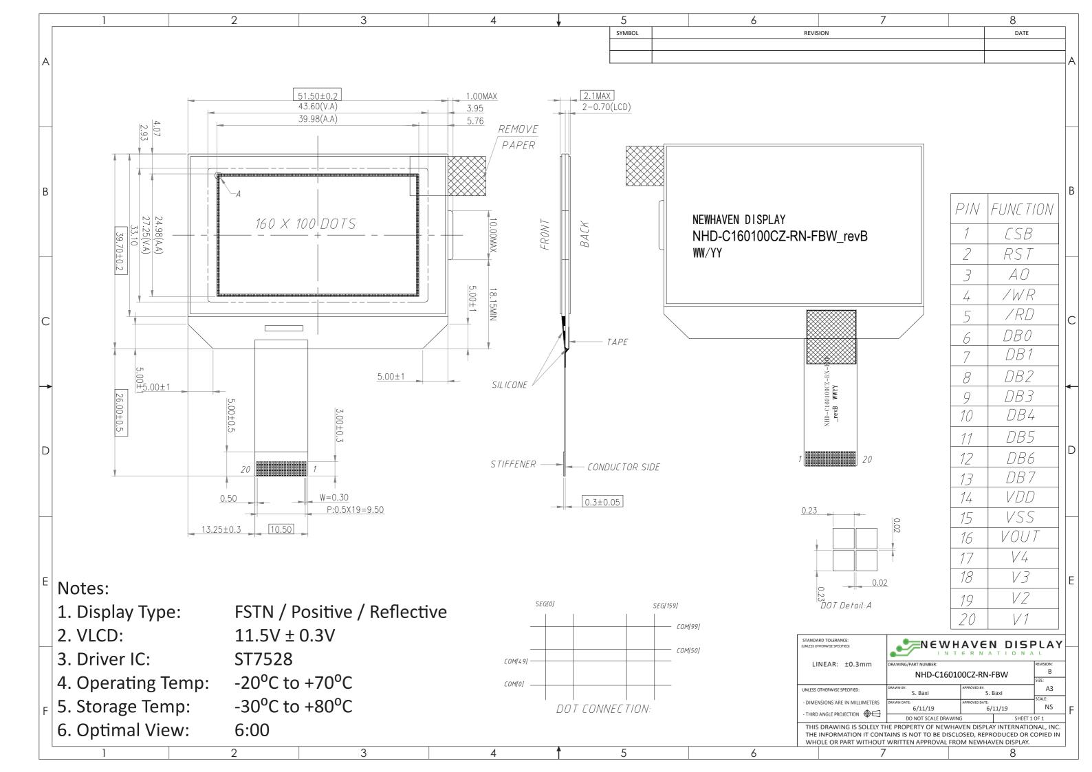
Pin Description and Wiring Diagram
