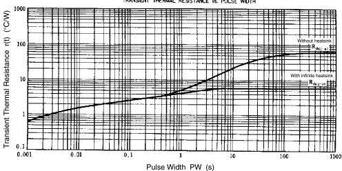
TRANSIENT THERMAL RESISTANCE vs. PULSE WIDTH
