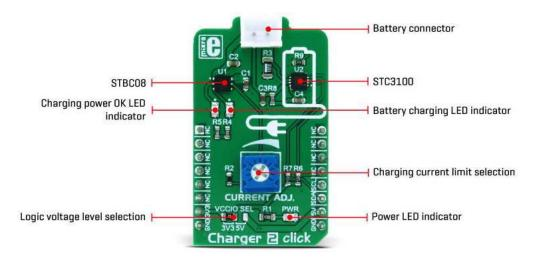
Two LEDs are used to signalize status of the STBC08 IC: red LED is used to signalize the ongoing charge process. The green LED signalizes if the charging conditions are nominal and within the specs. It signalizes the validity of the charging voltage value.
