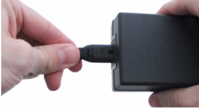
Figure 2.4 – Connect Power Supply and Adapter
