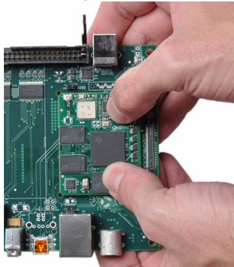
Figure 2.2 – Connect SOM-M2 to eXperimenter Baseboard
