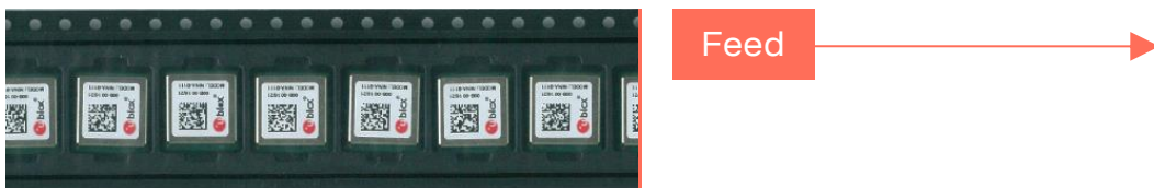
Figure 16: NINA-W101 module on tape orientation
