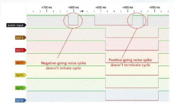
This logic analyzer capture of an LS10 series switch service cycle shows a noisy switch input commonly applied to all six device channels. Note the initial 19 ms low-going glitch at approximately +780 ms does not start a cycle, and the following 19ms high-going glitch at approximately +915 ms does not terminate the cycle. LS10 series devices are designed to function flawlessly in hostile electrical environments. These devices ignore any uninvited transitional pulses of < 20ms duration.
