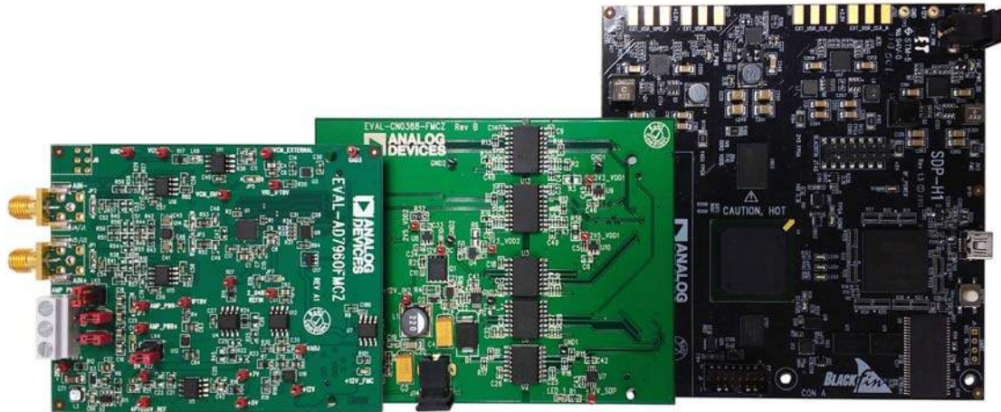
Figure 2. EVAL-AD7960FMCZ , EVAL-CN0388-FMCZ Isolator, and EVAL-SDP-CH1Z Boards Connected Together
