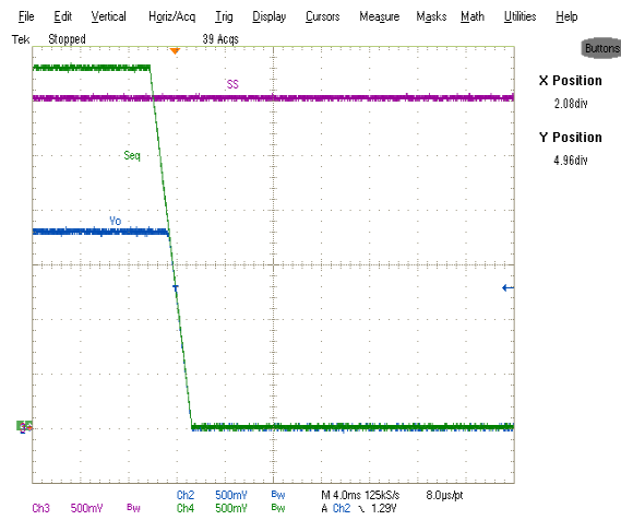
Fig. 25: Simultaneous Tracking a 3.3V input at power-up and shut-down Ch2: Vout (1.8V) Ch3:SS (1.8V) Ch4: Seq (3.3V)
