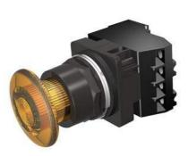
30mm BlackMax, Epoxy Coated Corrosion Resistant Complete Metal Unit Illuminated Push-Pull Operator Transformer type, 120V AC LED Lamp Mushroom Head Cap Small 1 3/4" (44.5 mm) Plastic, Amber 2 Position Maintained, Pull-to-Release with 1 N.O. - 1 N.C. Heavy Duty Contacts, A600/P600 UL Listed, CSA Certified NEMA 1,3,3R,4,4X,12,13 & Automotive Standards
