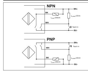
By means of the Teach-in wire, the functions described in the Teach-in Guide can be setup.
