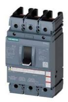
molded case switch 3VA5 UL frame 250 max short-circuit curr. rating 65kA a 480 V 3-pole MCS110, In=250A without overload protection SELF PROTECTION Ii=10 x In Al-lug, line side
