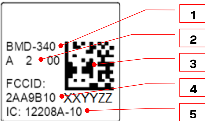
Figure 14: Module marking for type number BMD-340-A-R-01
