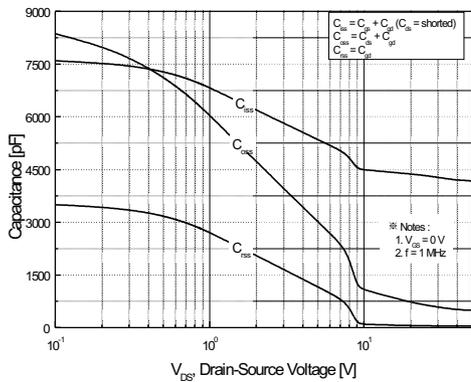
Figure 5. Capacitance Characteristics
