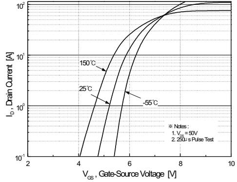
Figure 2. Transfer Characteristics
