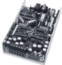
Output Rise Time: <250 ms (10% to 90%) Remote Sense Standard on V1 and V2
