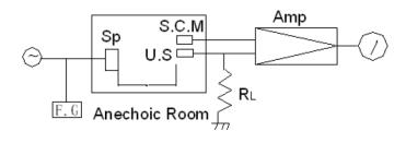
RL: 3.9K Ω U.S :Ultrasonic Sensor S.C.M:Standard Cappacitor Microphone Amp. :Ampifier OSC. :Oscillator Sp :Tweeter F.C :Frequency Counter
