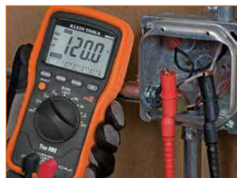
Alligator Clips Attach to Bare Wire
