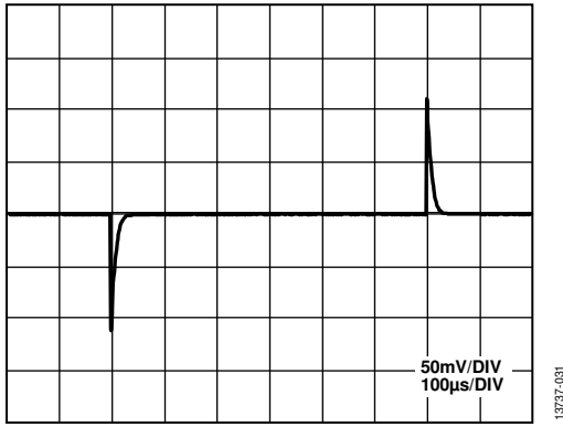
Figure 31. Load Transient Response (100 \mu A Load Change)
