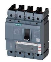
circuit breaker 3VA5 UL frame 250 breaking capacity class C 100kA @ 480V 4-pole, line protection TM210, FTFM, In=100A overload protection Ir=100A fixed short-circuit protection Ii=10 x In N conductor unprotected without connection
