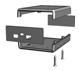
NOTE: ENCLOSURE SUPPLIED WITH 4 COVER SCREWS, ONLY 2 COVER SCREWS REQUIRED FOR ASSEMBLY
