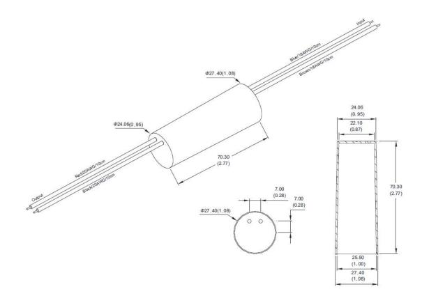
Dimensions mm (inch) Case Tolerance ±0.50 (±0.02)
