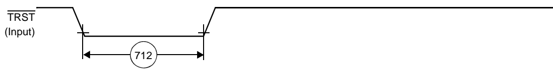
Figure 25. \overline{\text{TRST}} Timing Diagram
