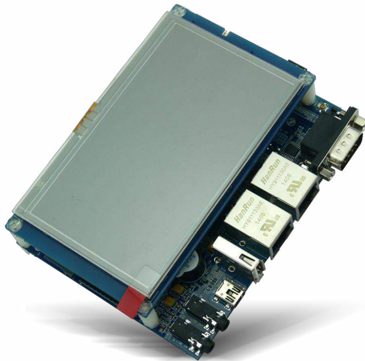
MYD-AM335X-Y Development Board with 4.3-inch LCD
