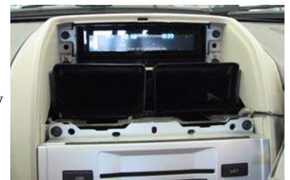
Air Vent Assembly Removed
