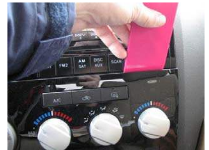
AC Bezel released w/ Dash Tool
