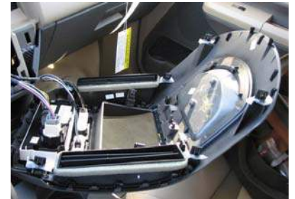
Radio Climate Control, Air Vent, Bezel Removed
