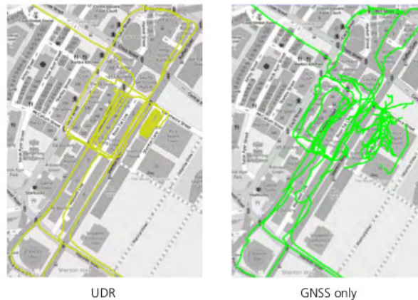
Untethered Dead Reckoning vs GNSS Only Comparison in an Urban Canyon. Image Courtesy of u-blox from the UDR Whitepaper.
