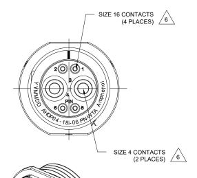
RECEPTACLE, 18-06 POS, PIN CONT., STANDARD DIA. SEAL, AHDP
