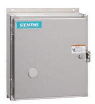
Non-reversing NEMA contactor, Size 4, Three phase full voltage, Contactor amp rating 135A, 3 wire (NO aux included), 24VAC 50-60Hz coil, Non-combination type, Encl NEMA type 4X 304 S-Steel, Water/dust tight noncorrosive, Extra-wide enclosure
