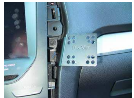
Mount installed showing screw location
