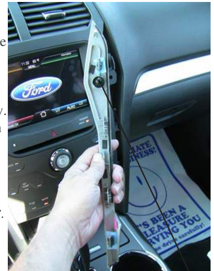
Bezel removal (plastic lug)
