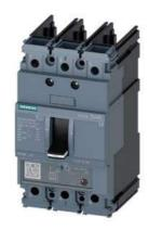
circuit breaker 3VA5 UL frame 125 breaking capacity class M 35kA @ 480 V 3-pole, line protection TM230, FTAM, In=15A overload protection Ir=15A fixed short-circuit protection II=5...10xIN UL 489 SB (naval), 50° cel. without connection
