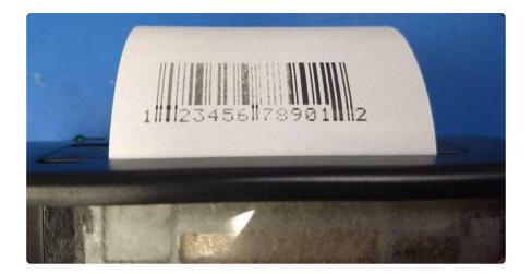
The first parameter to print\_barcode is a string that defines the barcode value (this varies depending on the type of barcode, a UPC A code is 13 digits). The second parameter is the type of the barcode, which again is dependent on the printer firmware. Typical values you might use include:
