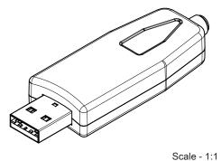
CHECKED REVISION DATE (YYYY-MM-DD) GENERAL TOLERANCE PROJECTION METHOD GE 001.011 2019-10-11 DIN ISO 2768-1m **WIRL-PR09 Telesto-III Plug** Würth Elektronik eiSos GmbH & Co. KG **Wireless USB stick 915MHz SMA** EMC & Inductive Solutions Max-Eyth-Str. 1 2609026291001 74638 Waldenburg Tel. +49 (0) 79 42 945 - 0 www.we-online.com STATUS BUSINESS UNIT PAGE 1/4 eiSmart Valid eiSos@we-online.com
