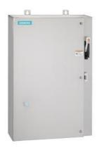
Non-reversing motor starter Size 1 Three phase full voltage Solid-state overload relay OLRelay amp range 0.25-1A Combination type 30Amp non-fusible disconnect Encl NEMA type 4X 316 S-steel Water/dust tight non-corrosive Extra-wide enclosure
