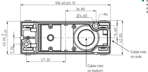
As an alternative to mounting with the metal clip, the bottom of the housing can be attached directly with M4 screws.
