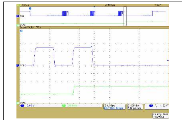
FIGURE 2-45: 10\text{ k}\Omega – Low-Voltage Increment Wiper Settling Time ( V_{DD} = 5.5\text{V} ) ( 1\ \mu\text{s}/\text{Div} ).
