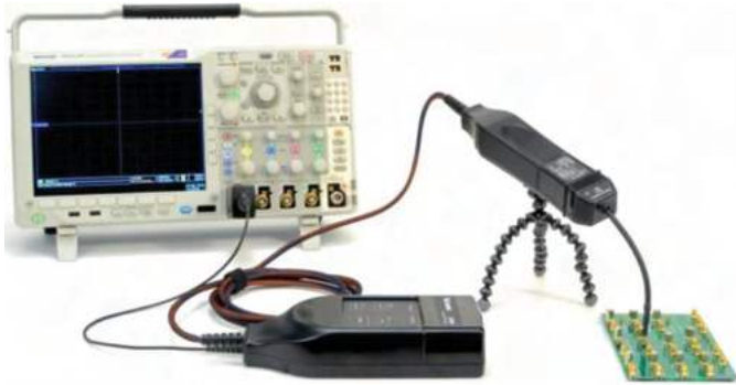
Figure 4: Tektronix IsoVu measurement setup.
