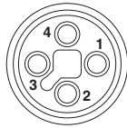
Connector pin assignment of M12 socket, 4-pos., T-coded, view of socket side
