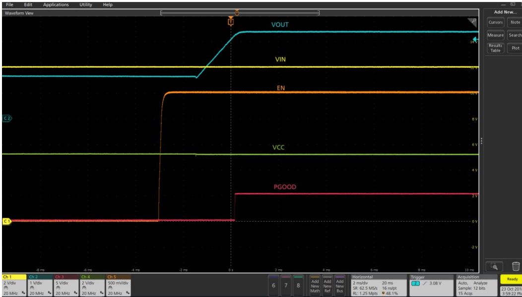
Figure 21 Startup into pre-bias (Ch1:PV IN , Ch2: V OUT , Ch3: PGood, Ch4:V CC , Ch5: Enable)
